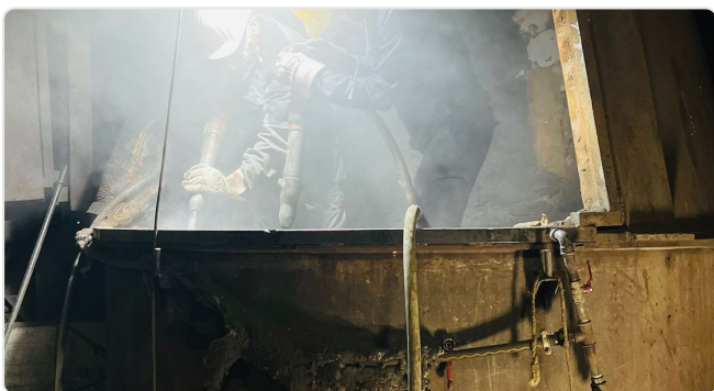
Lining on the cupola furnace
