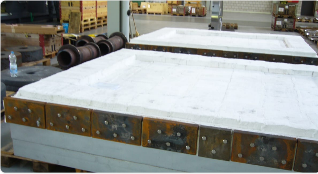
Fully lined lids in the workshop
