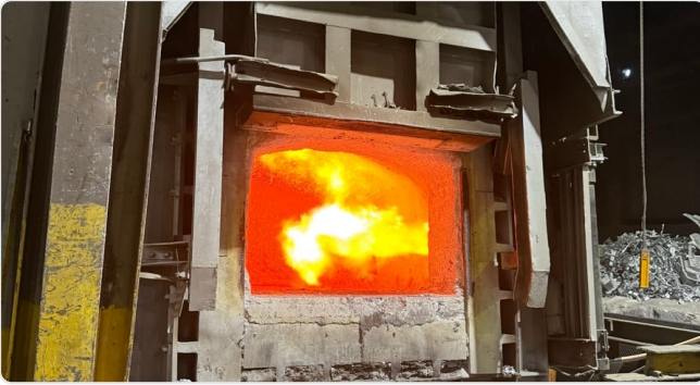
Flame in the furnace chamber — what matters is where it impinges
