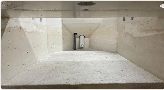
Dosing furnace: tight geometry, constant metal contact
